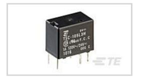
Contact Voltage Rating: 24 VDC Signal Relay Coil Power Rating (DC): 150 mW Isolation (HF Parameter): -20.7dB @ 900MHz, -39dB @ 100MHz Insertion Loss (HF Parameter): -.02dB @ 100MHz, -.27dB @ 900MHz
